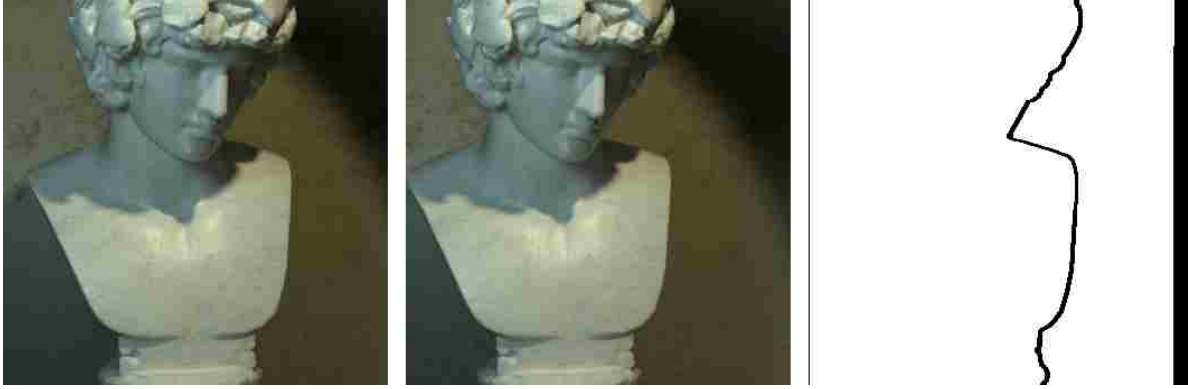
Figure 1.5: An example consistency mask (shown on the right) for the central view compared to an adjacent view (left and middle respectively).
